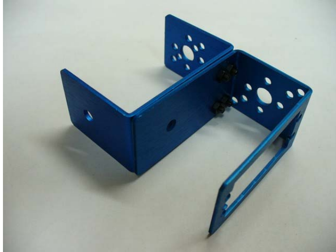
Figure 5 Two pieces of R-joint servo is connected with 4 pairs of nuts and bolts.
