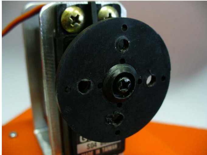
Figure 17 The servo motor #2 and its horn set piece are installed.
