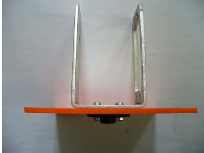
Figure 15 The horn set piece, the acrylic board and the U-Shape are attached together.
