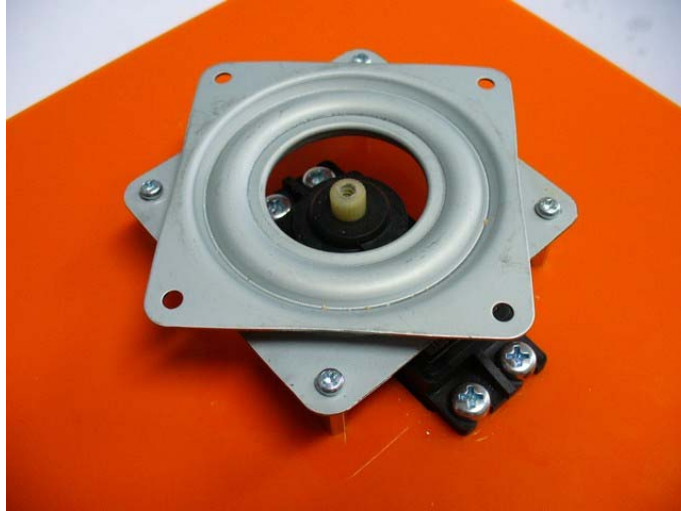
Figure 13 The ball bearing rotation plate is attached to the acrylic board.
