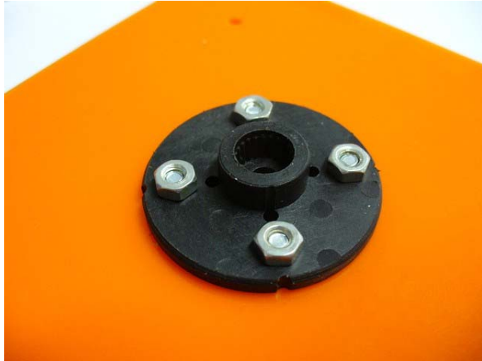
Figure 14 The drilled horn set piece after attached to the acrylic board
