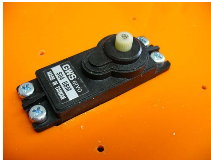
Figure 12 The servo motor #1 is attached to the acrylic board.
