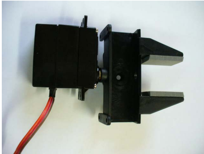
Figure 3 The servo motor #5 that used to rotate the gripper is installed
